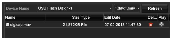
Figure 16-7 Local Upgrade Interface
