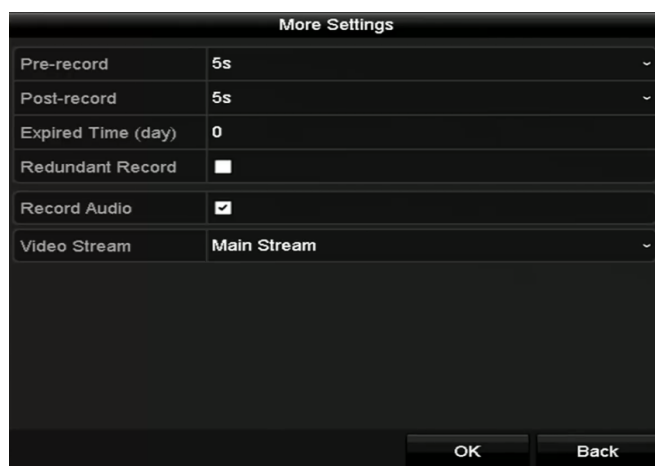
Figure 5-4 More Settings of Record Parameters
