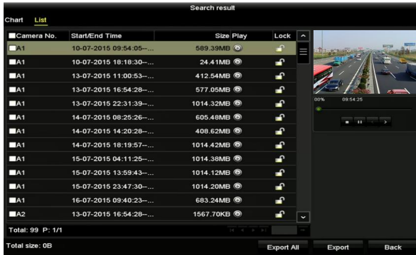
Figure 7-2 Result of Normal Video Search for Backup
