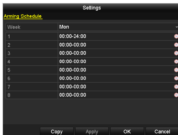
Figure 8-22 Set Arming Schedule of Alarm Output
