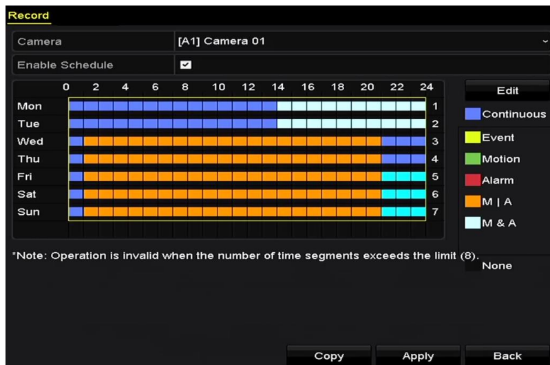
Figure 5-12 Draw the Recording Schedule
