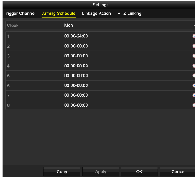
Figure 8-8 Set Arming Schedule of Alarm Input
