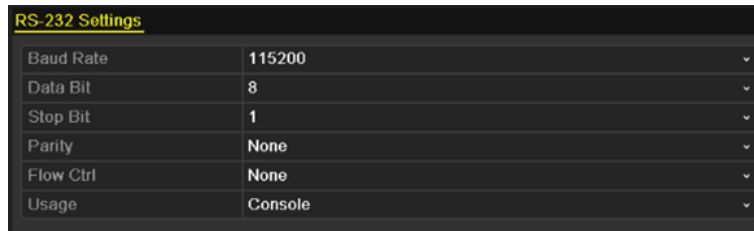
Figure 17-3 RS-232 Settings Interface
