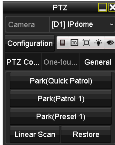
Figure 4-12 PTZ Panel - One-touch
