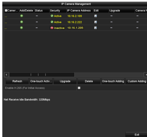
Figure 2-35 IP Camera Management Interface
